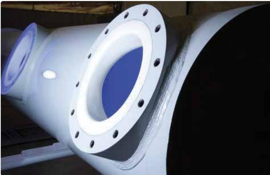
*Diameter changes, wall penetrations and gussets that spanned the ID had to be protected with a uniform and uninterrupted bonded liner of modified HDPE.*
