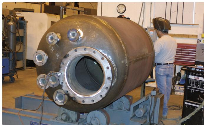
*On-site construction of steel vessel to ASME code*
